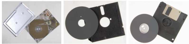
Images of the internal components in various magnetic disks: 1. Hard drive; 2. Floppy disk; 3. Floppy diskette
