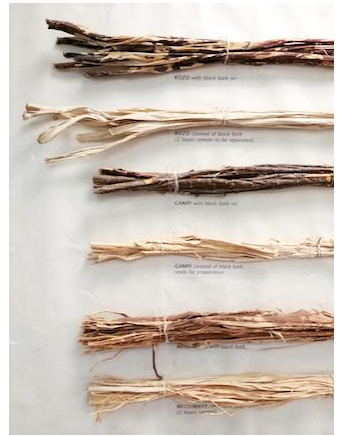
Japanese washi papermaking fibres (from top): 1&2 Kozo; 3&4 Gamp; 5&6 Mitsumata. Image: https://printdayinmay.com/2019/04/04/which-washi-choosing-japanese-paper-for-printmaking/
